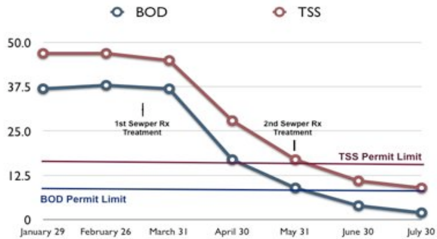
Figure 1 - Rosethorne effluent BOD/TSS reduction by Sewer Rx.
